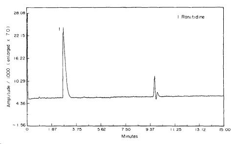
Figure 3 Direct analysis of Zantac syrup. Operating conditions: 20 mM sodium citrate (pH 2.5), V = 30 kV,  $T = 30^{\circ}\text{C}$ , UV detection at 210 nm,
