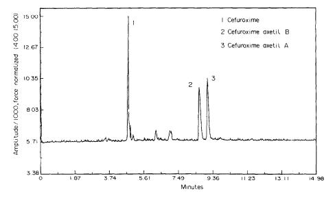
Figure 1 Degraded cefuroxime axetil sample analysis by MECC. Operating conditions:  $0.01 \text{ M Na}_2\text{HPO}_4$ ,  $0.06 \text{ M Na}_2\text{B}_4\text{O}_2$  and 0.05 M sodium dodecyl sulphate, V = 10 kV,  $T = 30^{\circ}\text{C}$ , UV detection at 276 nm.
