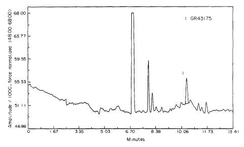
Figure 4 Analysis of 1  $\mu$ g ml<sup>-1</sup> GR43175 in urine. Operating conditions: 20 mM sodium citrate (pH 2.5), V = 11 kV, T = 25°C, UV detection at 210 nm.
